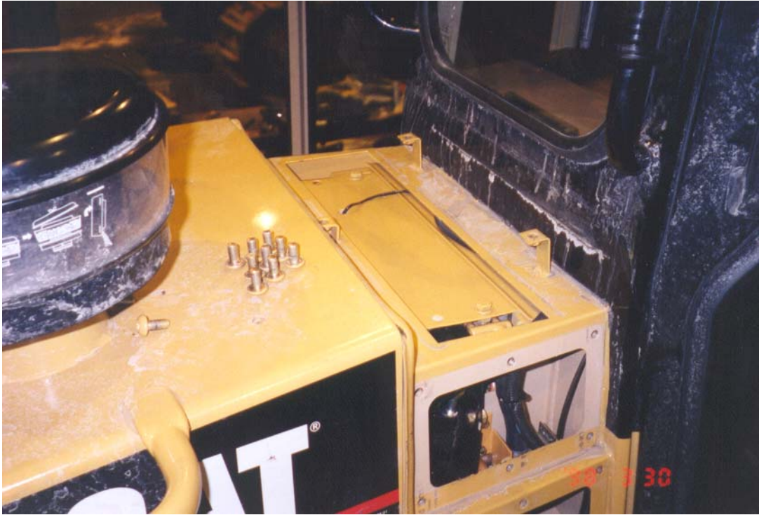
Evaporator cover in place with thermostat.
