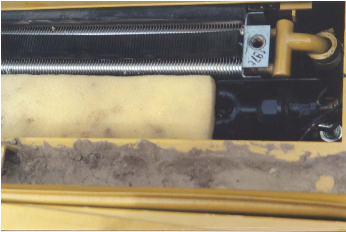
Top of evaporator assembly in heater box.
